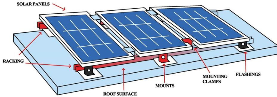
Fig.3.10.2. Rooftop solar installation components. (Source: own elaboration).
