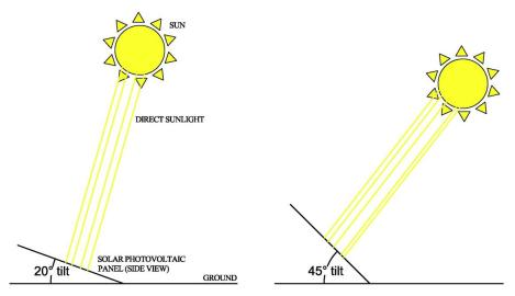
Fig.3.10.3. Solar panel tilt angle. (Source: own elaboration).
