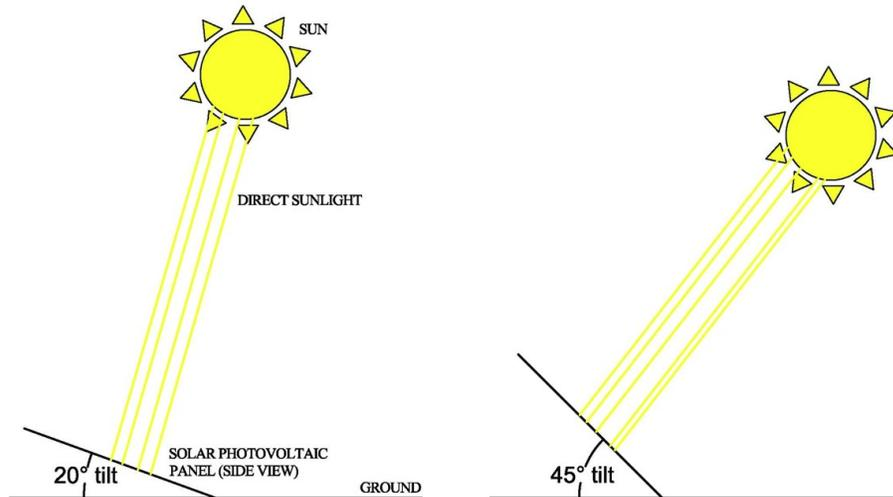
Fig.3.10.3. Solar panel tilt angle. (Source: own elaboration).
