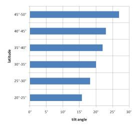
**Fig.3.10.4.** Solar panel tilt angle based on latitude. (Source: own elaboration baced on Sandhu, J., 2022)
