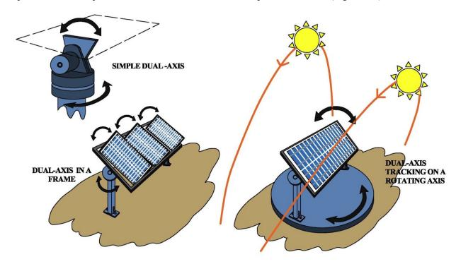
Fig.3.10.1. Dual-axis solar panel. (Source: own elaboration).
