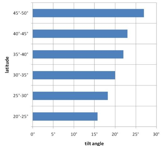
Fig.3.10.4. Solar panel tilt angle based on latitude. (Source: own elaboration based on Sandhu, J., 2022)
