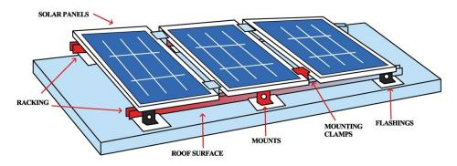
Fig.3.10.2. Rooftop solar installation components. (Source: own elaboration).
